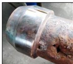
This time the problem was the main steam pipe at the top of the boiler, which required a major strip-down of the front end of the boiler and removal of the rusted pipe and fittings. This has had to be re-fabricated by an engineering company and we are now awaiting delivery of this part so that re-assembly of the loco can be finished.
